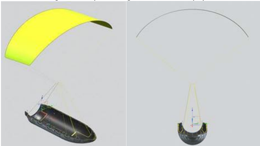
Figure 2-10. Payload Fairing Half with Parafoil Deployed
