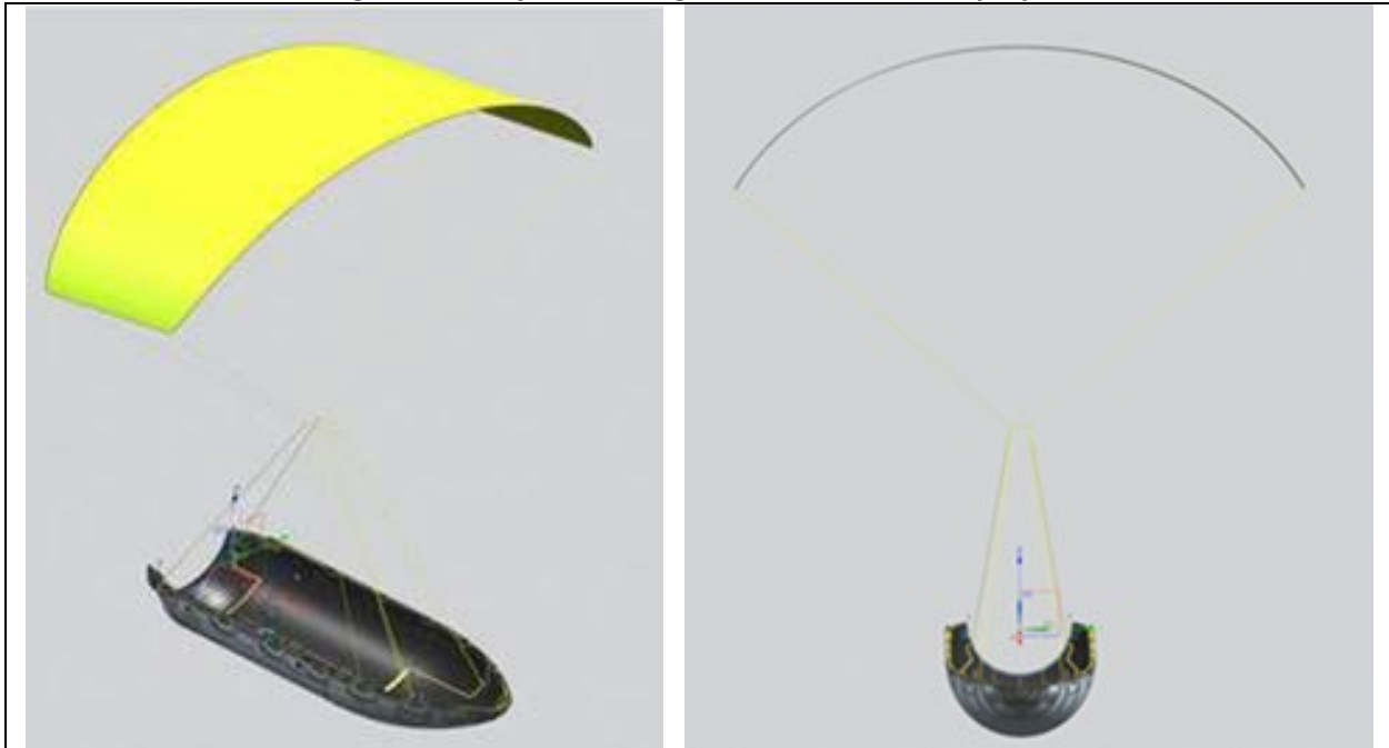
Figure A-3. Payload Fairing Half with Parafoil Deployed
