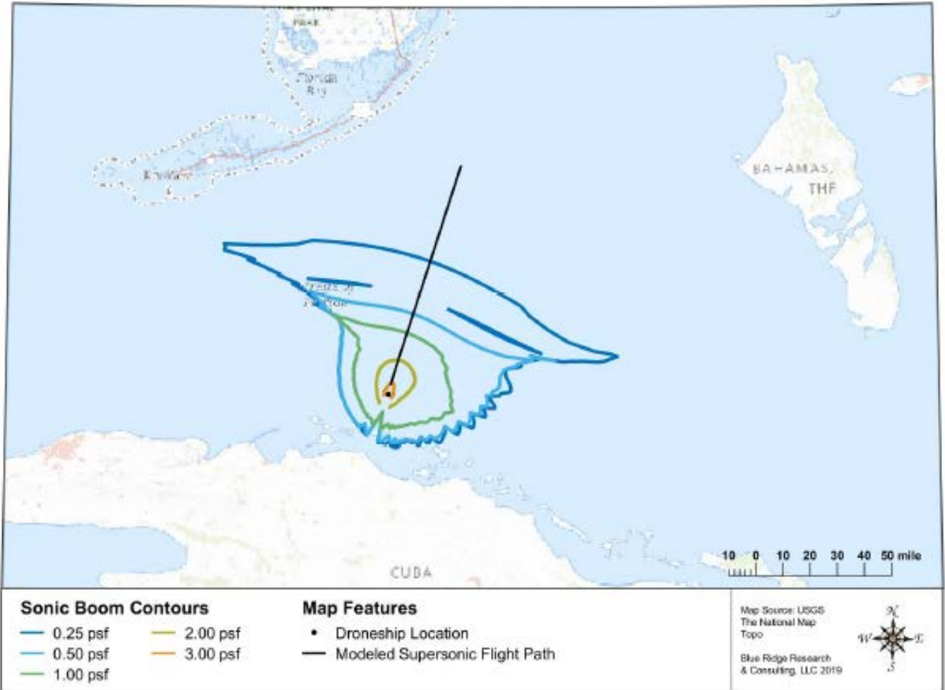
Figure 4-6. Predicted Sonic Boom Overpressure Contours for a Western Falcon 9 Drone Ship Landing
