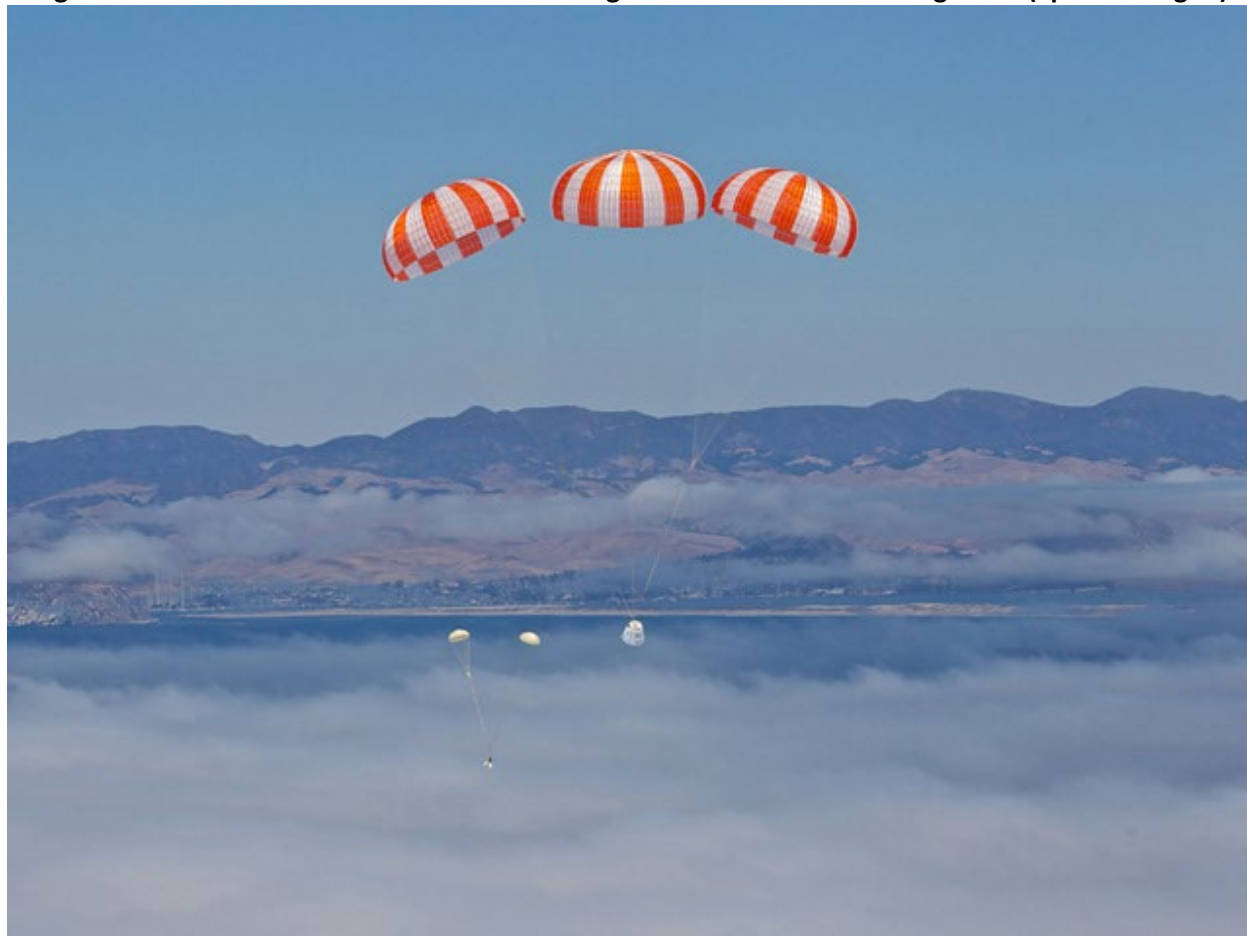
Figure A-1. Main Parachutes with Released Drogue Parachutes in the Background (SpaceX Dragon)
