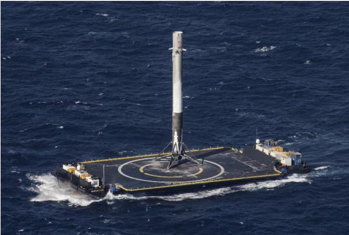
Figure 3-11. Image of the Booster Landing successfully landed on the droneship, the proposed methodology to be utilized for the Exuma sound mission (Provided by SpaceX).
